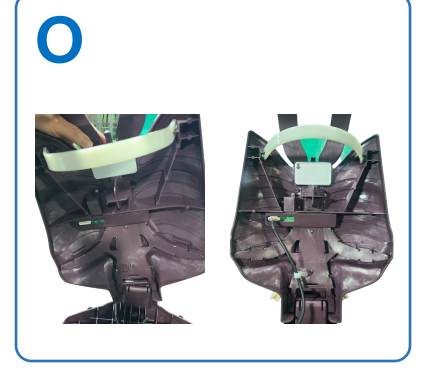
O. Connect the assembled rib frame to body frame and attach connector and clamp.
