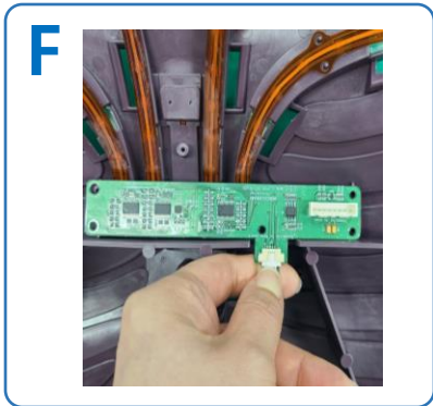
F. After removing the rib frame cover, remove rib board screw and detach the sensor connector.
